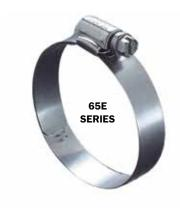
Lined clamps are specially designed for use with silicone rubber and other soft hose applications. The liner protects the hose surface and prevents it from extruding or shearing through the band notches as the clamp is tightened.
